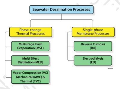
Figure 1 Commercial desalination processes
