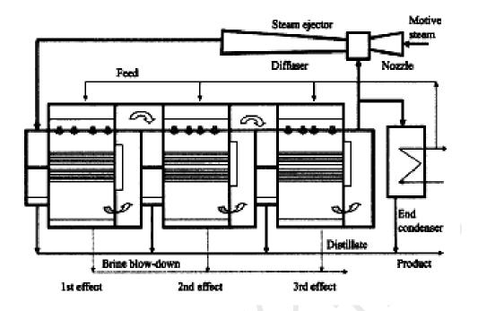
Figure 5 Multi-effect thermal vapor compression desalting unit
