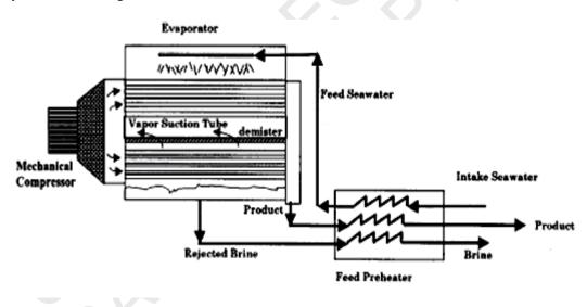
Figure 4 Mechanical vapor compression (MVC) process
