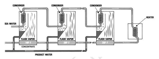
Figure 2 MSF process flow diagram
