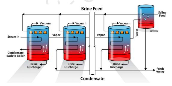
Figure 3 MED process flow diagram
