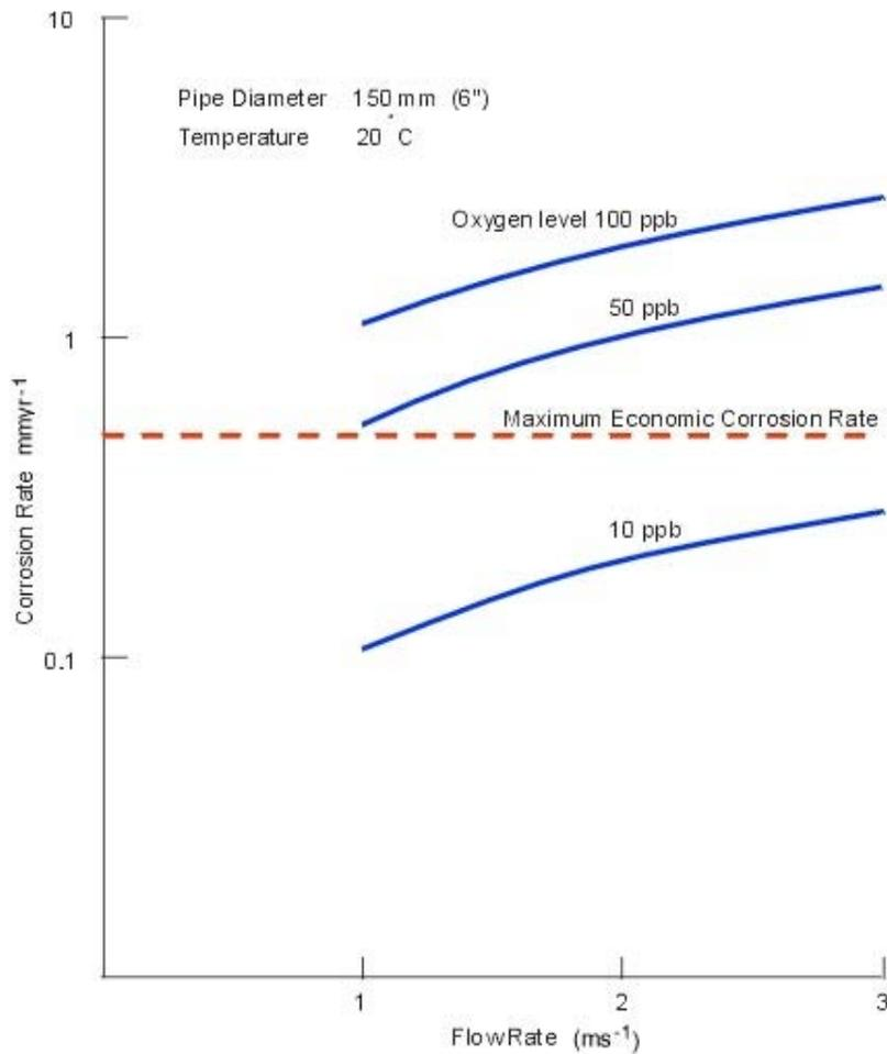
Figure 2. Estimates of corrosion of carbon steel in sea water as a function of flow rate at various oxygen concentrations.
