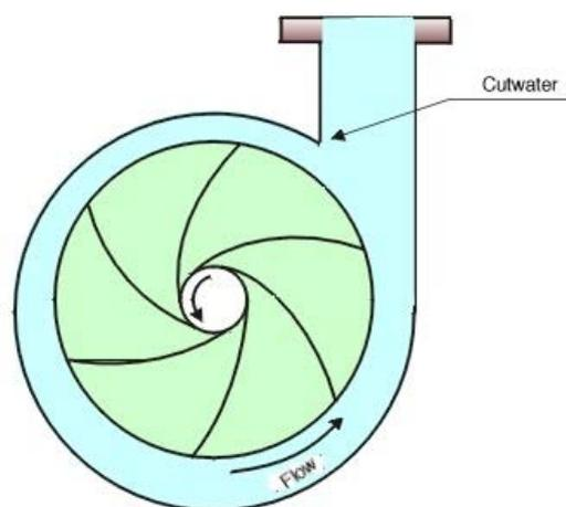
Figure 1. A simple impeller/casing arrangement.
