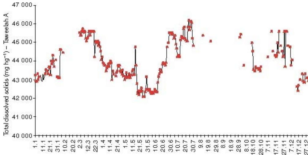
Figure 3. Typical total dissolved solids content of seawater at Plants 6 and 7 intake.
