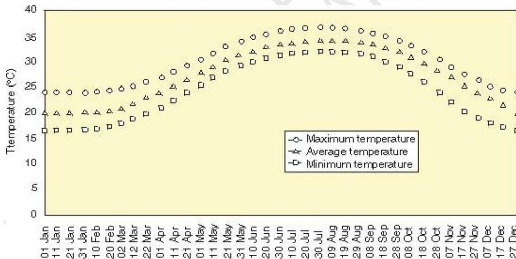
Figure 2. Typical seawater temperatures at Plants 6 and 7 intake.
