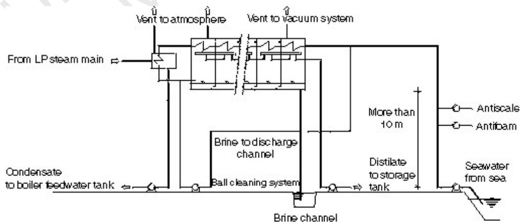
Figure 4. Flow scheme of a once-through multistage flash plant.
