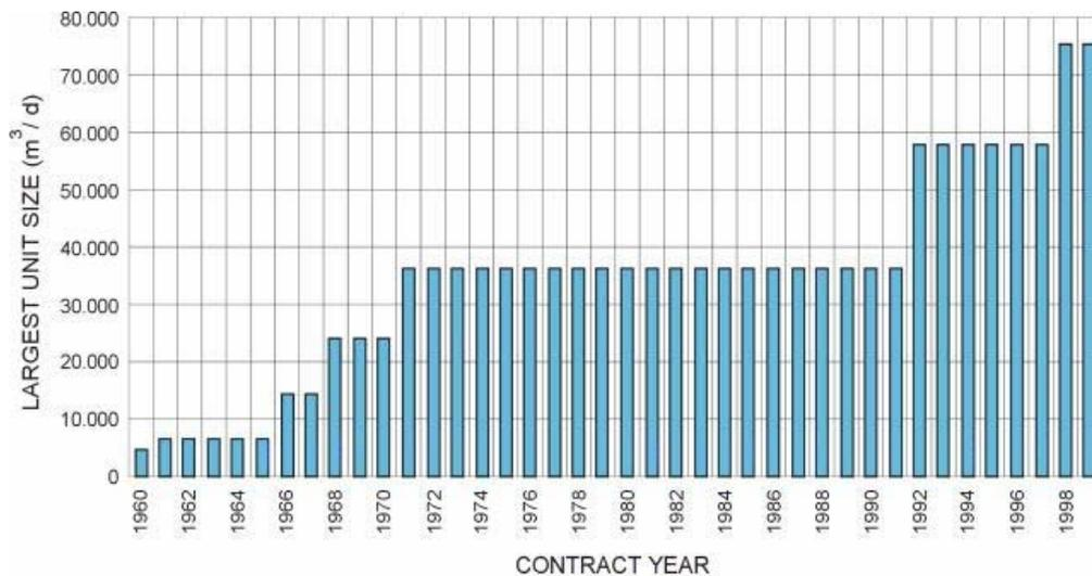
Figure 1. Development of multistage flash train sizes.
