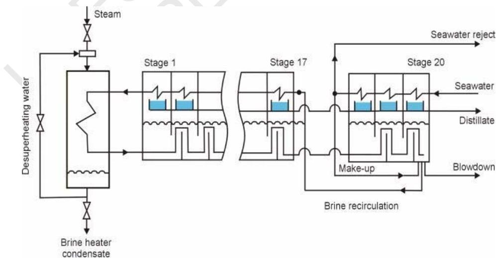
Figure 1. Schematic of 20 stage MSF desalination unit.
