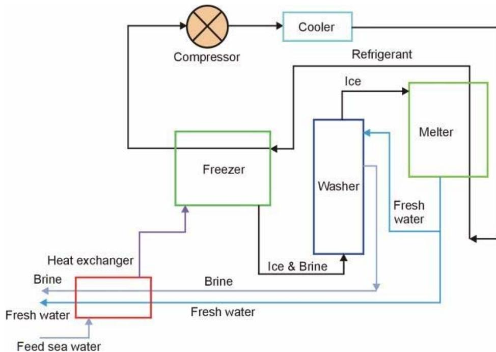
Figure 1. An indirect freezing process.
