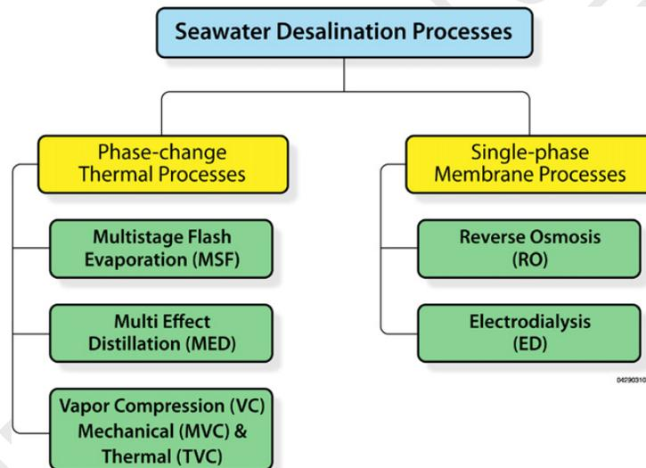
Figure 1 Commercial desalination processes
