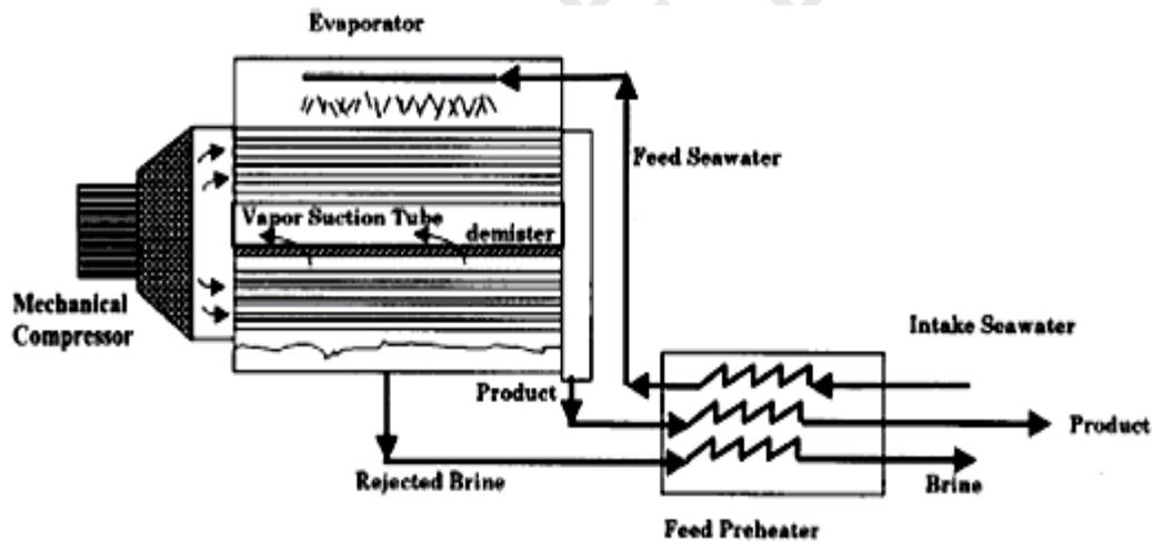
Figure 4 Mechanical vapor compression (MVC) process
