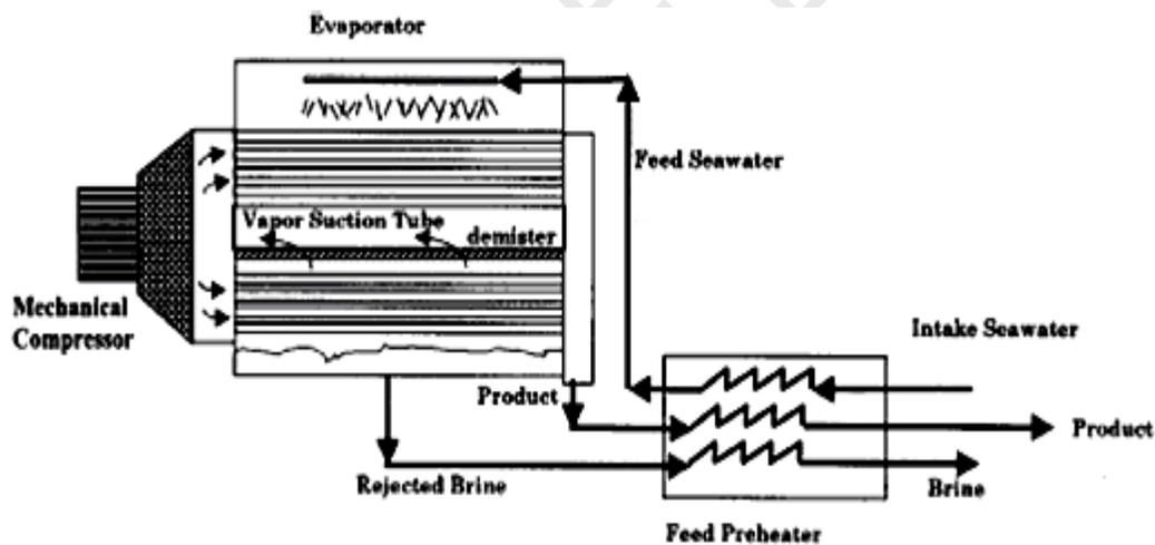
Figure 4 Mechanical vapor compression (MVC) process
