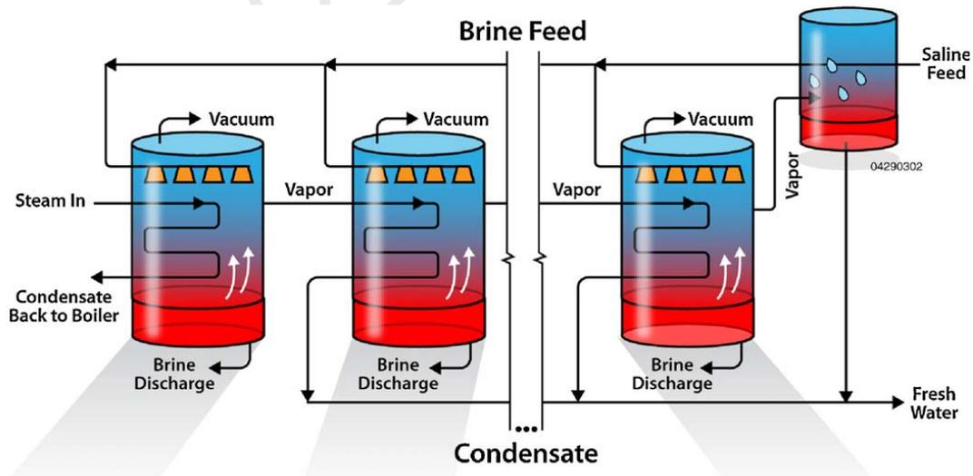
Figure 3 MED process flow diagram
