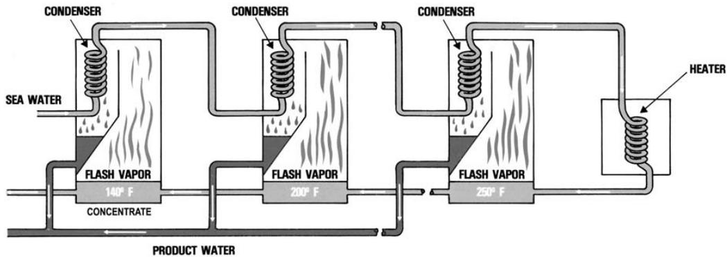
Figure 2 MSF process flow diagram
