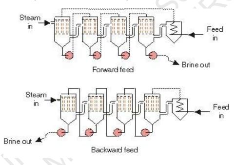
Figure 1. Types of feed for vertical tube evaporators.
