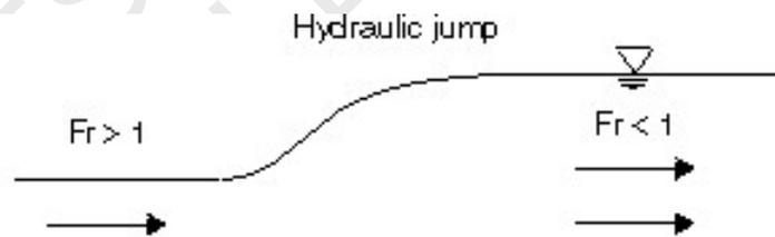
Figure 2. Transition from supercritical flow (hydraulic jump).
