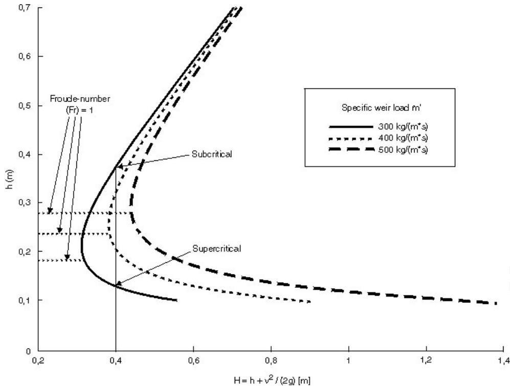
Figure 1. Influence of weir load and water level energy height.
