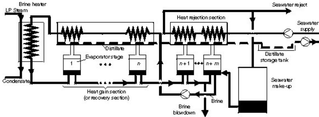
Figure 2. Schematic diagram of an MSF desalination Plant.
