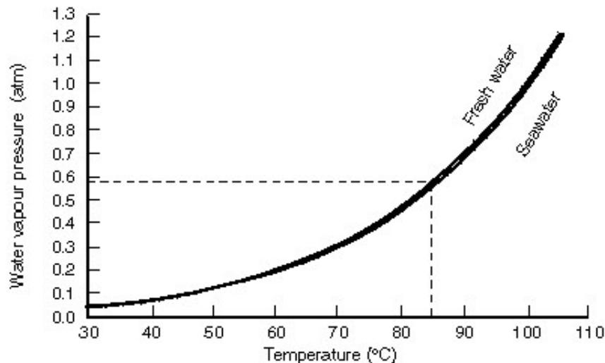
Figure 1. Increase of water vapor pressure of pure water and of seawater with temperature.
