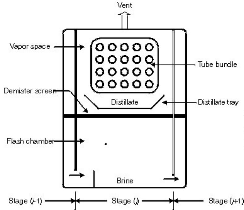
Figure 3. Cross section through a single distillation stage.
