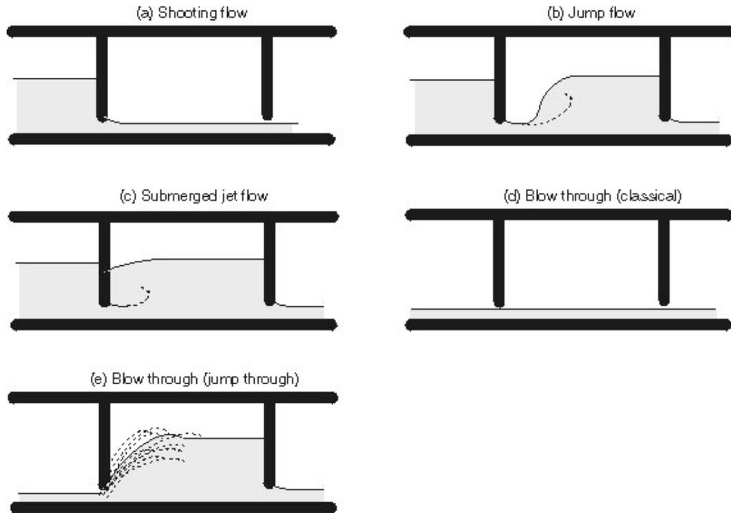
Figure 1. Conceivable single phase and blow through flow regimes in MSF plants.
