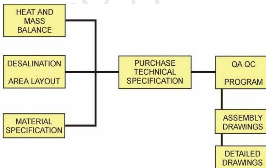
Figure 2. Schematic engineering activities sequence for auxiliary equipment procurement.
