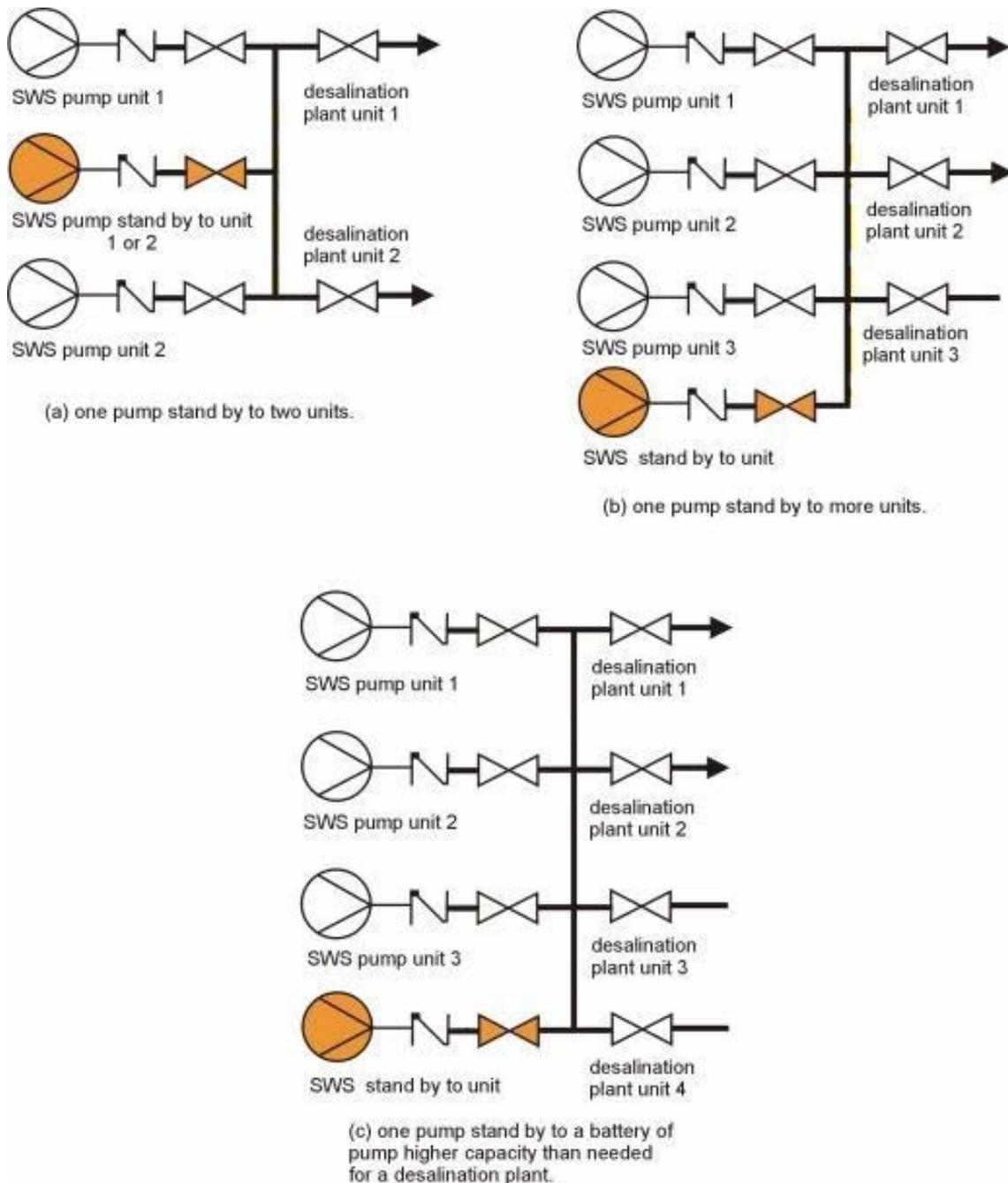
Figure 1. Stand-by criteria for sea water supply pumps.
