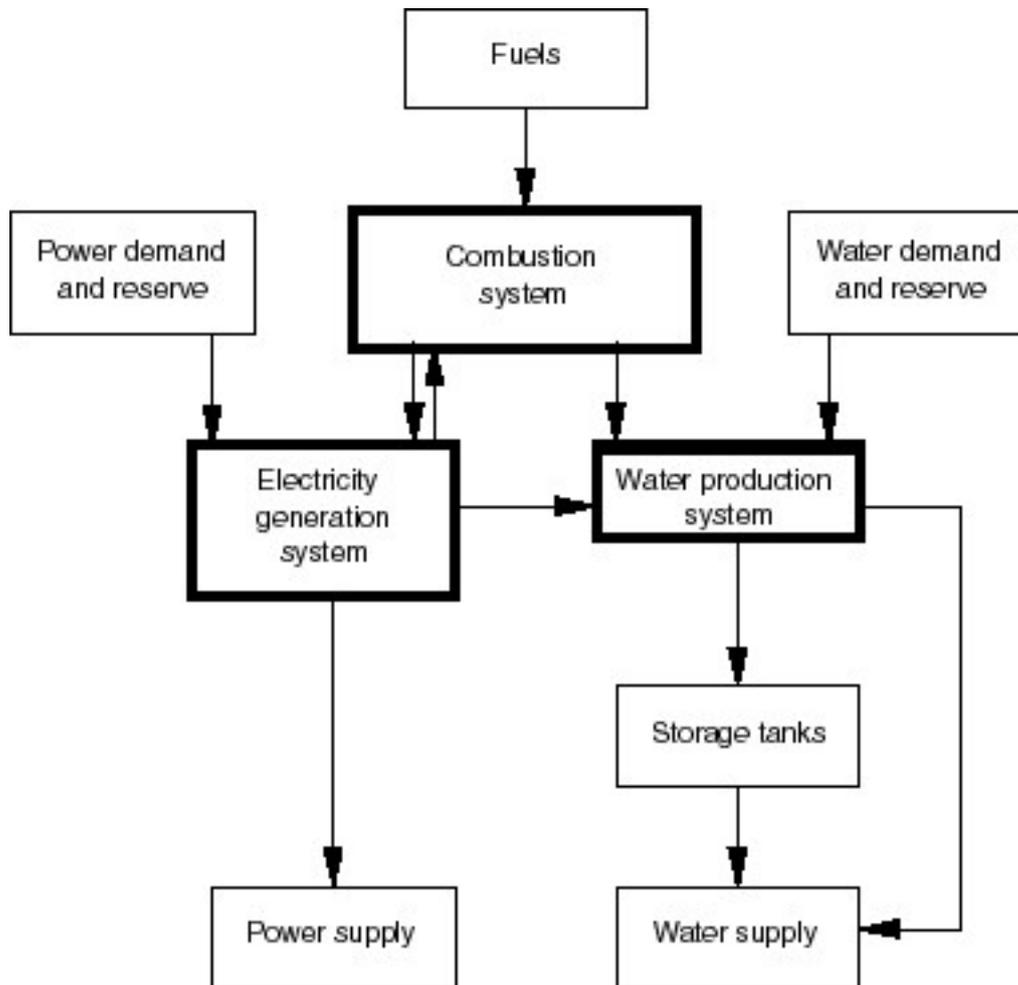
Figure 2. Structure of cogeneration system.
