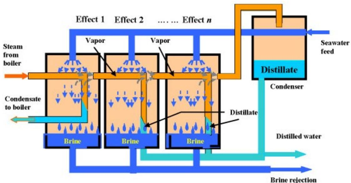
Figure 3. Schematic diagram of multi-effect distillation (MED) desalination system
