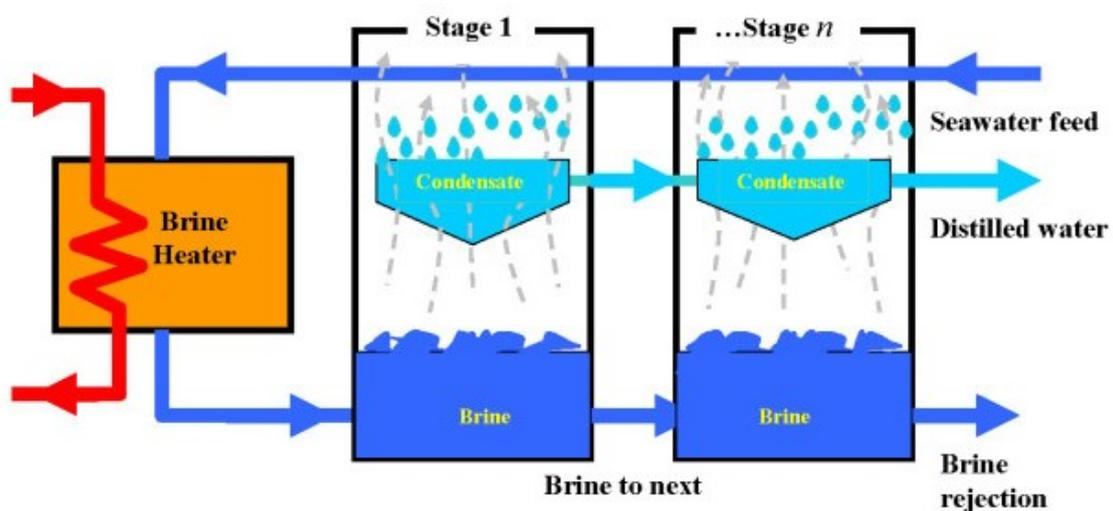
Figure 2. Schematic diagram of multi-stage flash (MSF) desalination system
