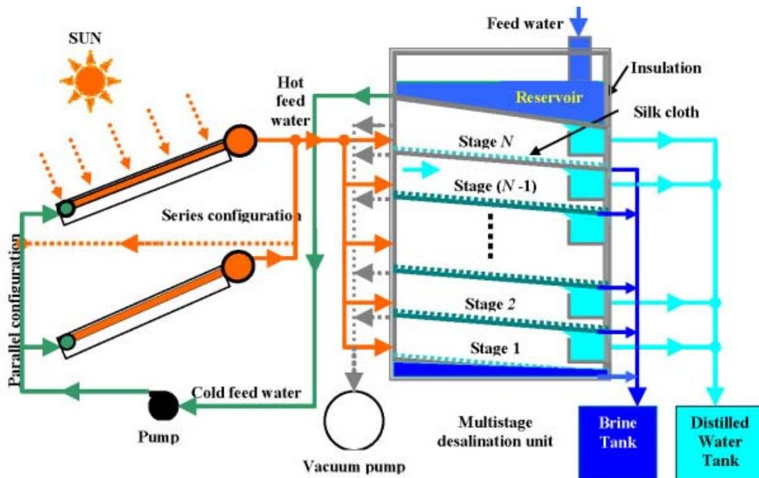
Figure 5. Multi-stage desalination unit with feed water flow coupled with solar flat plate collectors.
