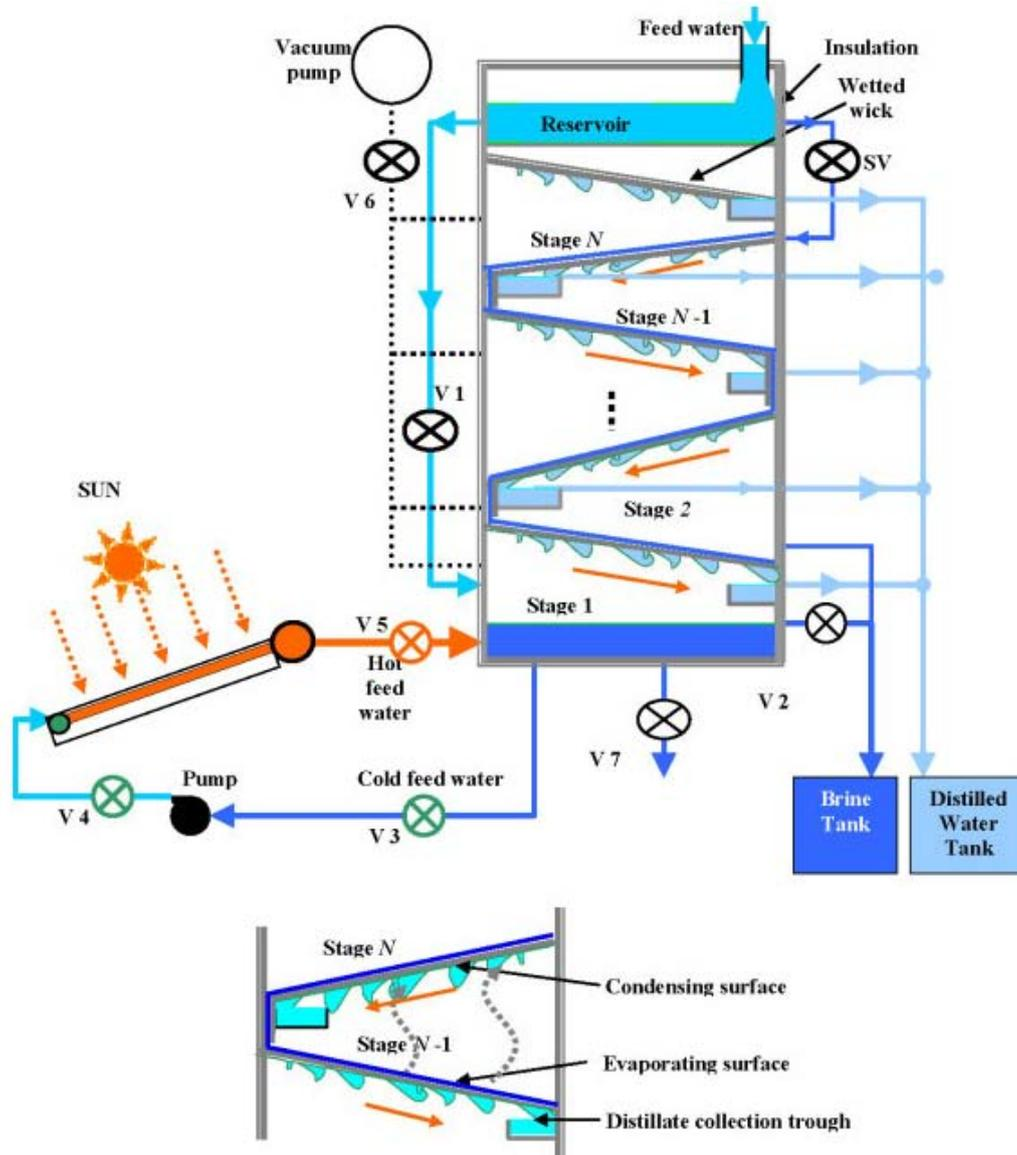
Figure 7. Active multistage series flow solar distillation unit analyzed by (Reddy and Sharon, 2017).
