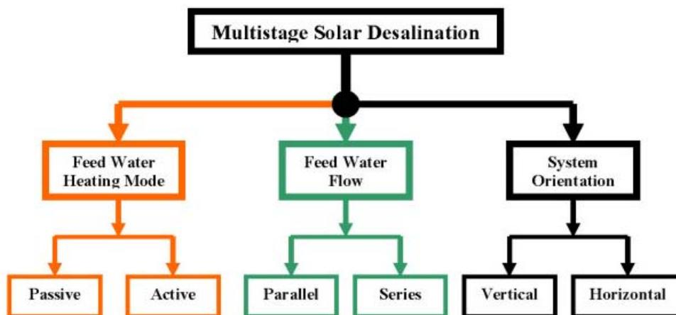
Figure 4. Classification of multistage solar desalination systems
