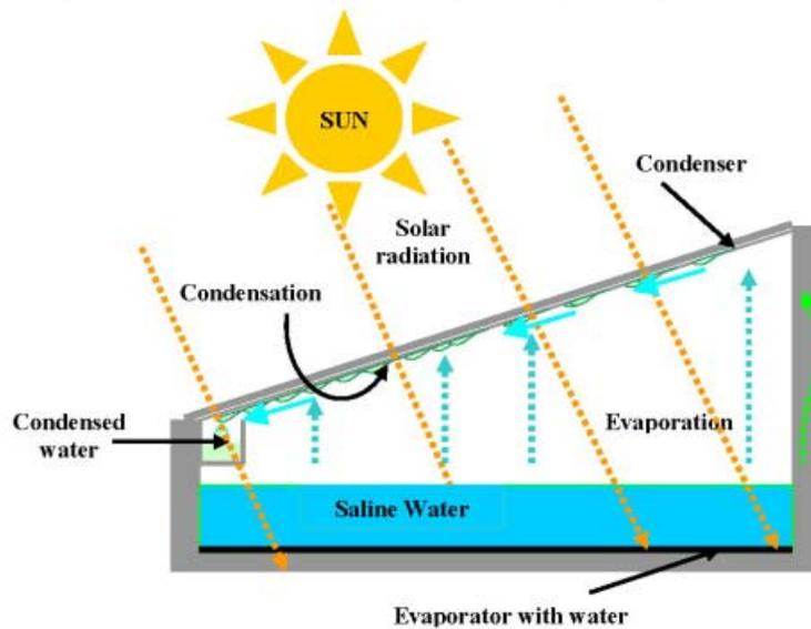
Figure 3. A schematic of solar thermal desalination working principle
