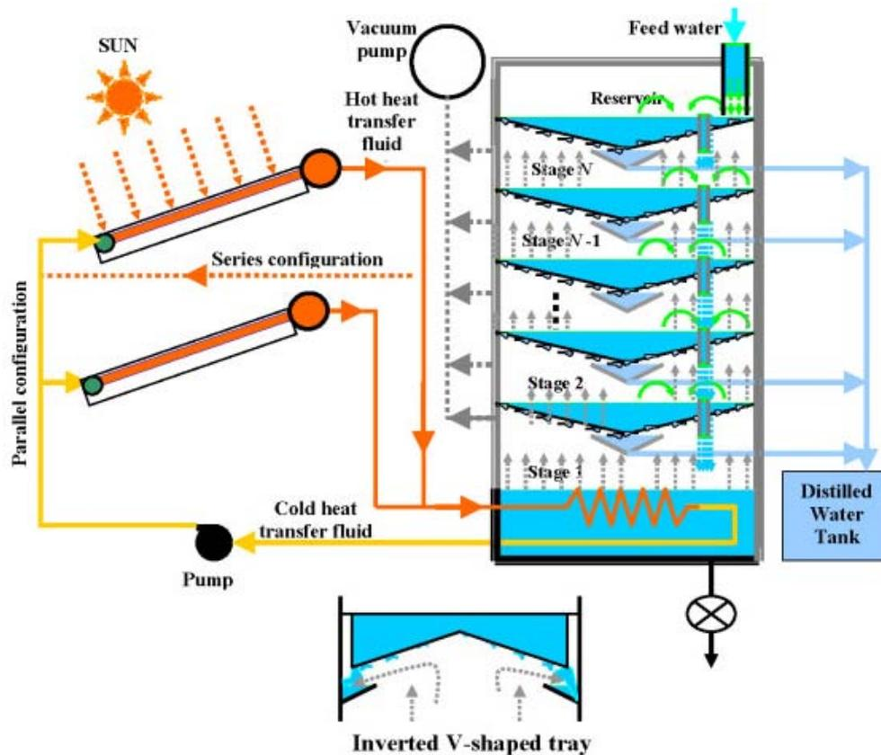
Figure 6. Multi-stage desalination unit with stagnant feed water level coupled with solar flat plate collectors and an alternate inverted V-shaped tray.
